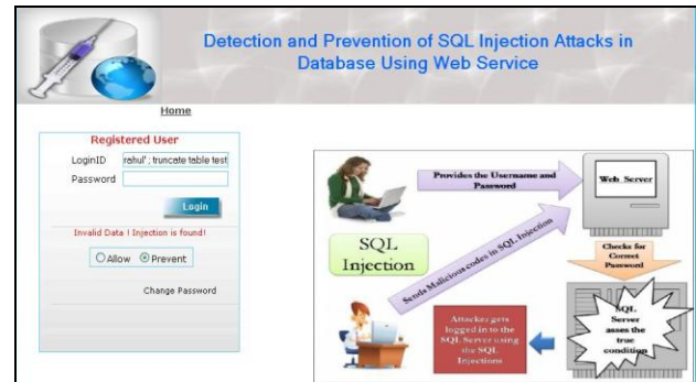
Figure 9: Piggybacked Attack Detected and Prevented Successfully
