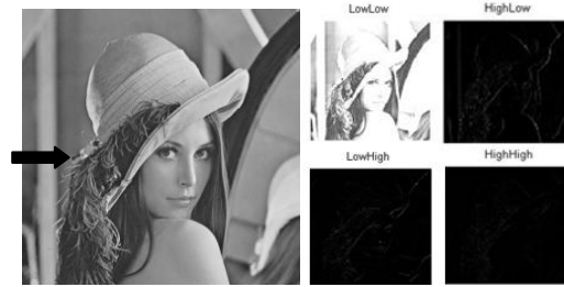
Fig. 2 Input image with different sub-bands after applying DWT
