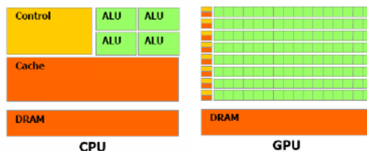
Figure 2 Architecture difference between CPU and GPU[3]
