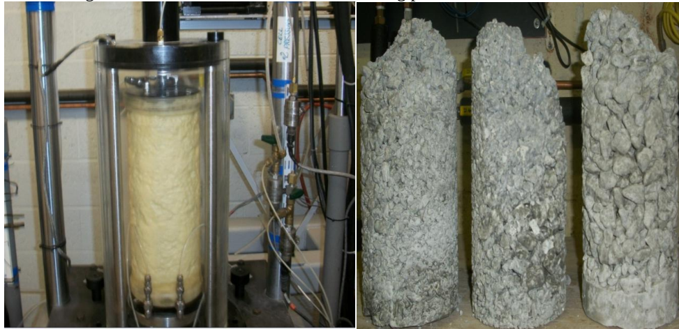
Measuring the K of CTPB using flexwall permeameter
