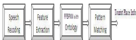
Figure 2. Block diagram of Odia key word based speech recognizer
