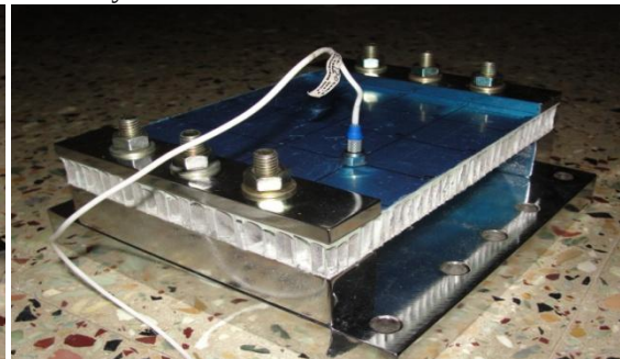
Fig. 2 Experimental setup for C-F-F-F condition
