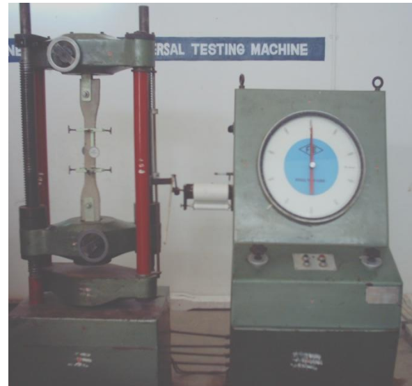
Plate 2. Tension test specimen in UTM
