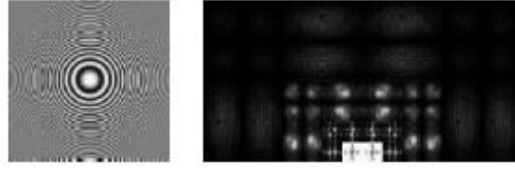
Figure 3 Left: isotropic test image containing various scale information, right: magnitude of its complex wavelet transform at level 3 showing both directional and scaling properties
