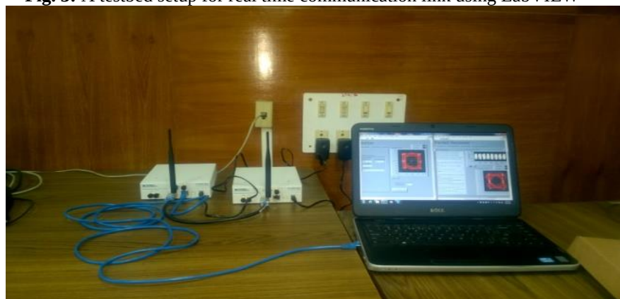
Fig. 3: A testbed setup for real time communication link using LabVIEW
