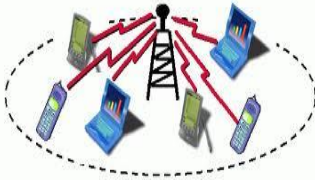
Fig. 1a: An Infrastructured Network
