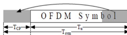
Fig.1 Cyclic prefix generation
