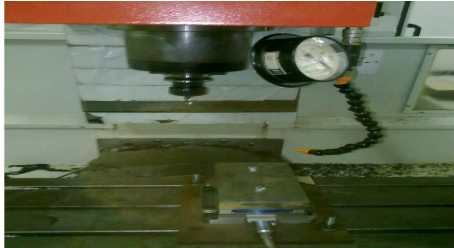
Figure 2 Dynamometer beneath workpiece and pressure gauge
