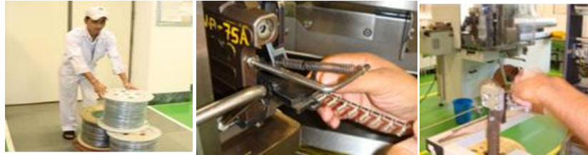
a. Material receiving b. wire feed in machine c. Terminal feed in machine (Problem)
