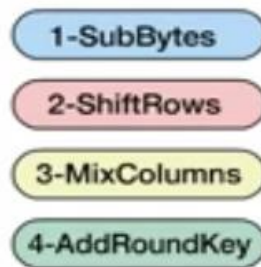
Figure. 1 Steps Used In Data Processing Unit Of AES
