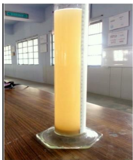
Fig 1 Settling of effluent after treatment
