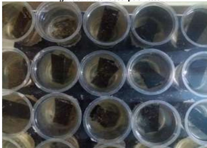
Figure 3. Water absorption test
