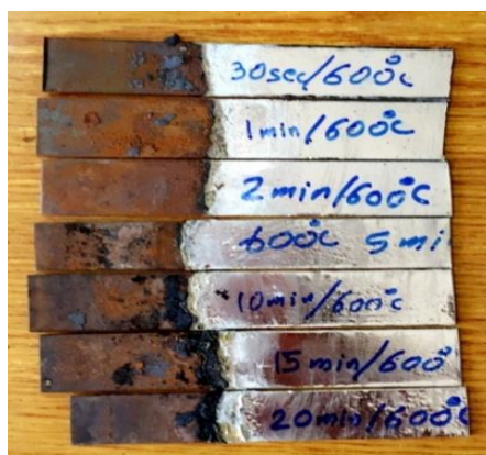
Figure (1) the specimens of steel after completed galvanizing process
