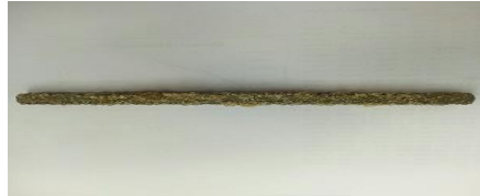
Figure 2. Sand-coated Hybrid FRP bar
