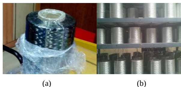
Figure 1. (a) Raw Carbon and (b) Glass fibres Rovings
