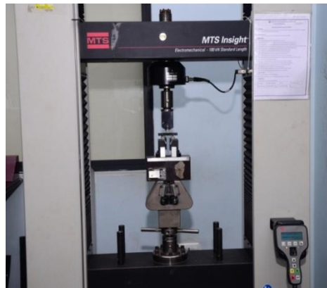
Fig.6. Short beam shear test setup
