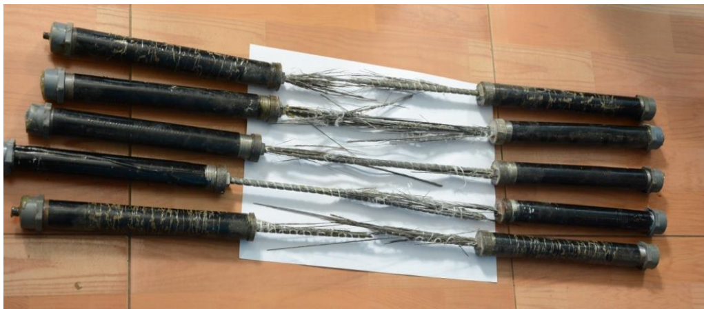
Fig.10. Failure of tensile specimens
