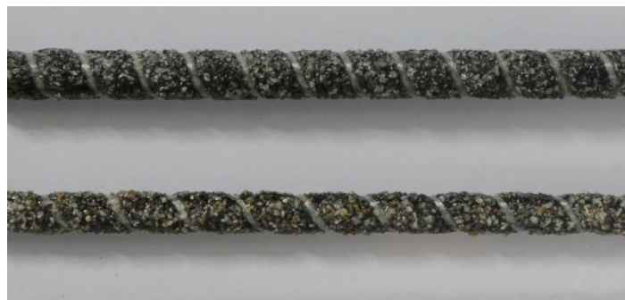
Fig.1 Sand-coated BFRP bars
