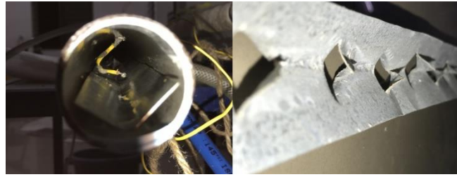
Fig. 2.2: Fabricated Strip and its Insertion inside the Tube
