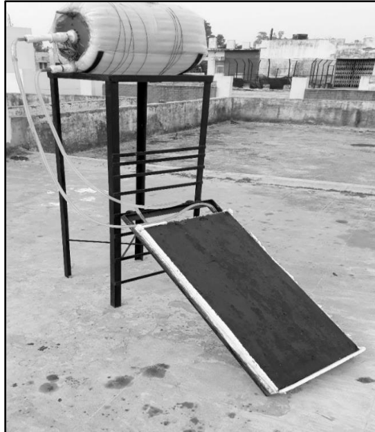
Figure 2: Concrete Slab Solar Water Heating System
