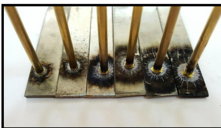
Figure (4), joining of pin in 30 degree head shape to plate in rang (40-90) volt.
