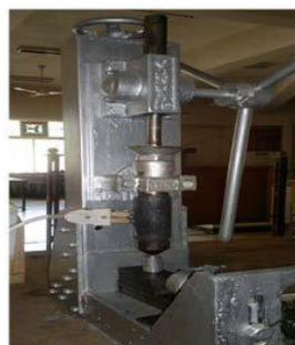
Fig. 3 Injection moulding machine with Stainless steel mould
