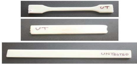
Fig. 4 Plain ABS test specimens
