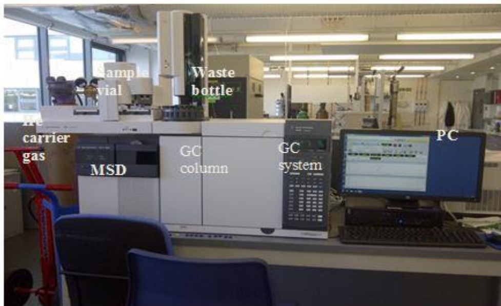
Fig. 2: Agilent 7890B autosampler Gas chromatography (GC) system coupled with Agilent technologies 5977A mass spectrometry detector (MSD) at the Centre for Process Integration and Membrane Technology (CPIMT), RGU.
