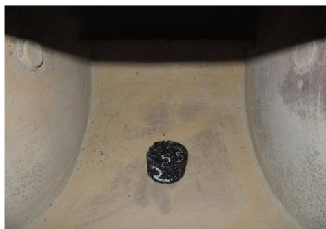
Figure 4 Unaged PFC specimen subjected to Abrasion Test
