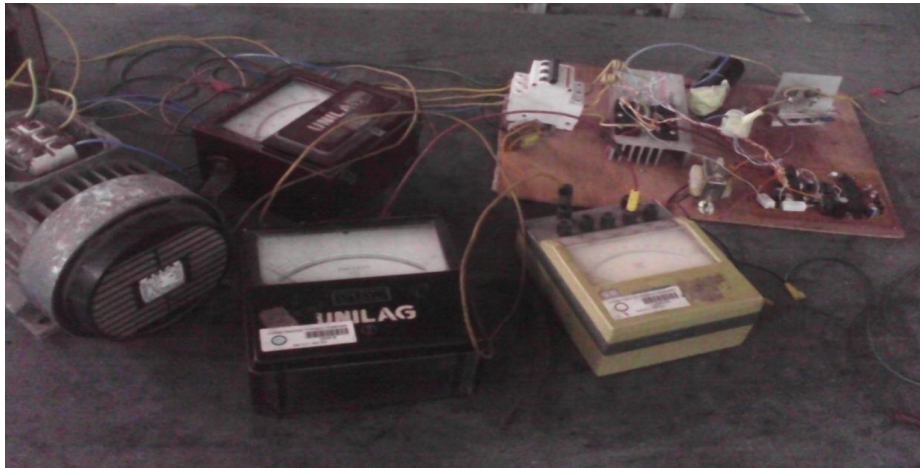
Figure 7 Test Rig with Controlled 3-Phase Induction Machine and the Inverter Controllers
