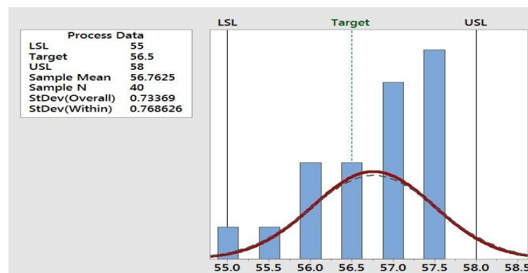
Figure 4: Histogram of Hardness of Rod before Improvement
