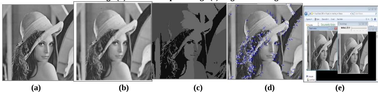
Figure 5: (a) Original Lena.jpg (512x512 size) (b) Filtered image at 80% noise density (c) Segmented image (d) SIFT descriptor image (e) Registered Image
