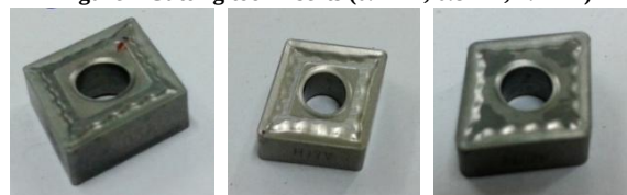
Figure 2 Cutting tool-inserts (0.4mm, 0.8mm, 1.2mm)
