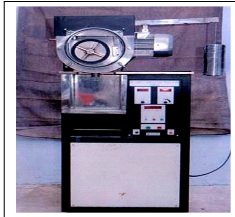
Figure 2 Photograph of the slurry abrasion test apparatus
