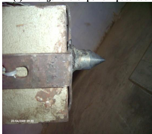
(a) Arrangement for point impact load
