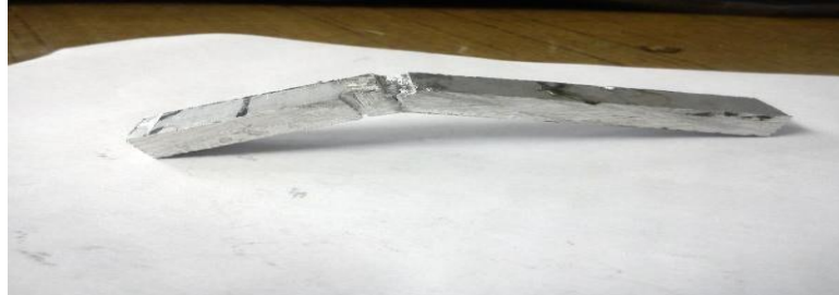
Fig 5 Image showing breaking of sample from notch after impact test
