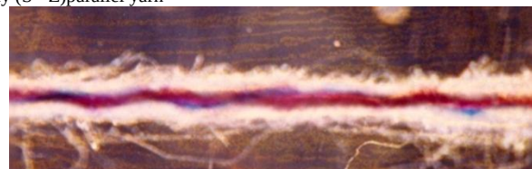
Fig. 6 b. Twist distribution in parallel yarns (Z + Z)
