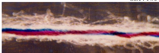
Fig. 6 a. Twist distribution in parallel yarns (S + S)
