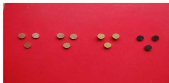
Picture: 12 Sintered pellets heat treated at 500°C in hydrogen atmosphere for 30 minutes.
