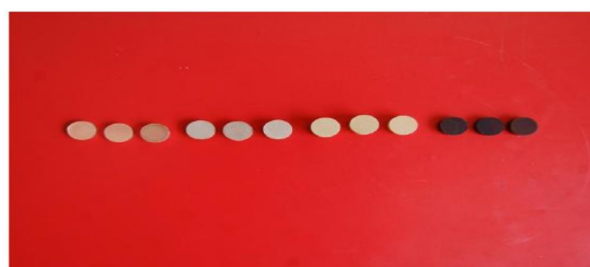
Picture: 11 Green pellets (as mixed, 2hr, 20hr and 48 hr milled samples) prepared in hydraulic press with application of 5 ton load)
