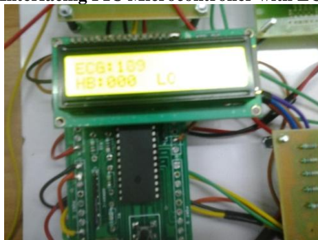
Figure 4 Interfacing PIC Microcontroller with LCD display
