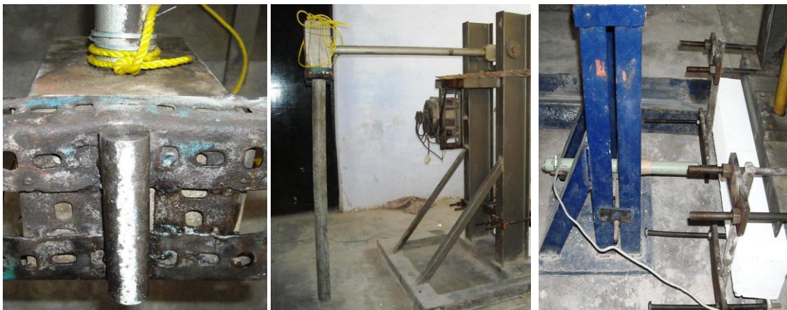
Figure 1 Testing of beam under line impact load
