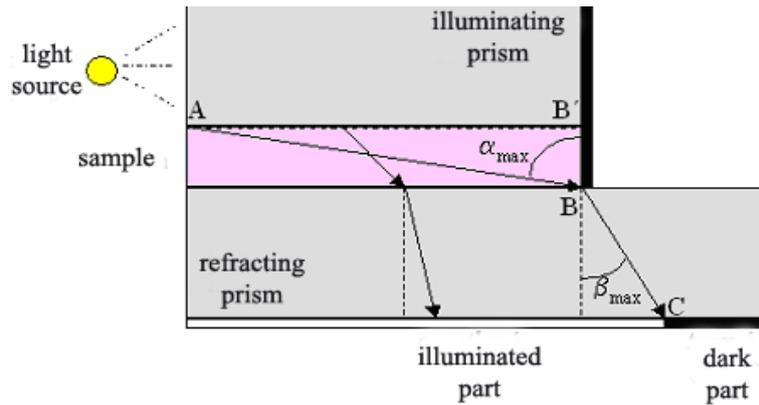
Fig 1- Schematic diagram of Abbe Refractometer
