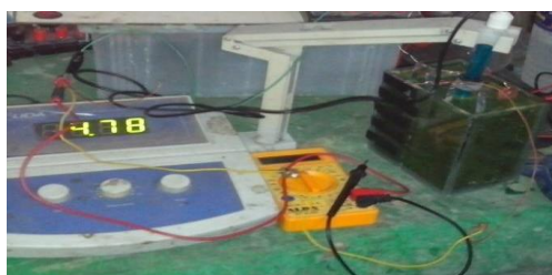
Figure 4 An experimental set-up of studying the self-discharge characteristics of BPL cell.
