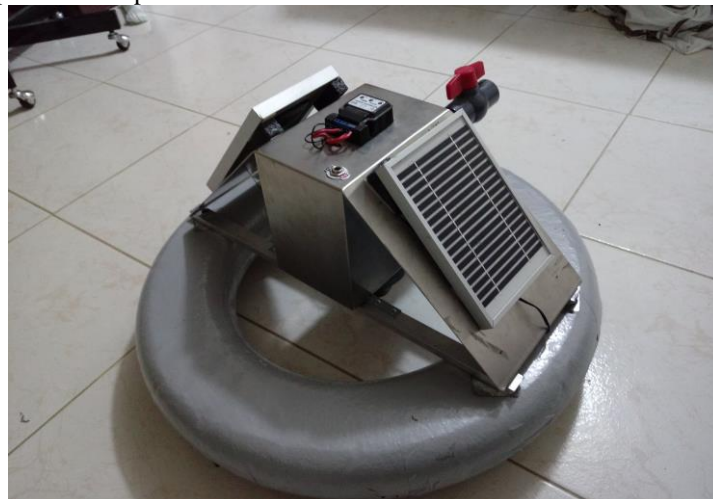
Figure 3: Fully fabricated solar powered floating pump
