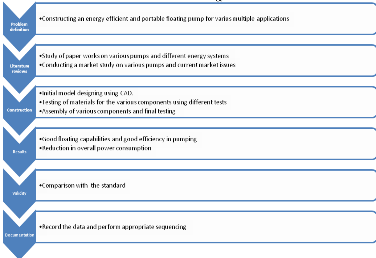
Figure 1: Methodology involved in the design and fabrication of floating pump
