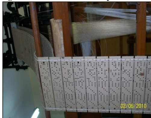
Figure 4: Strand of cards with punched holes
