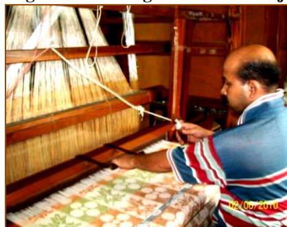
Figure 2: Weaving of fabric using handloom with jacquard facility
