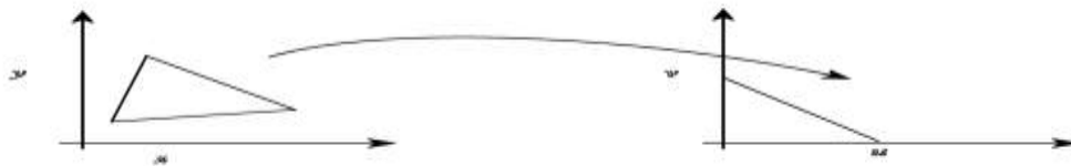
Figure (2) showing transformation of arbitrary triangle in to unit right angled triangle
