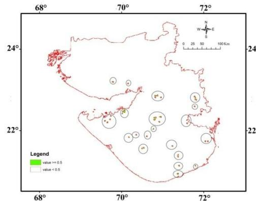
It is known that 1 MW PV plant requires approximately 5.3 acres of area. On this basis, the area of the potential sites can be calculated from which the size of PV plants can be computed. The details of these findings and their description are presented in table 2.
