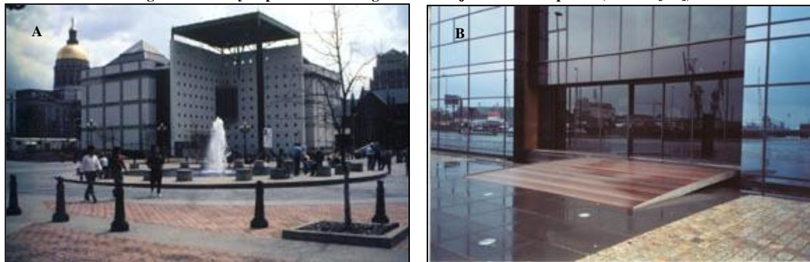
Fig . 8 :This entrance in Fig . 8aThe fountain and high canopy in front of the building clearly mark the entrance,This entrance in Fig.8b is virtually impossible to distinguish from adjacent window panels (Source: [ 14])
